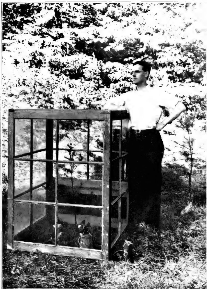
FUMIGATION CHAMBER FOR TESTING EFFECTS OF SULPHUR DIOXID ON YOUNG TREES.
